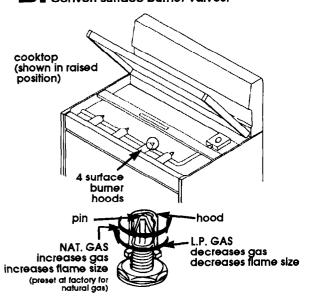
1. Lift and lock cooktop in up position. 2. Use 1/2" wrench to turn hood clockwise until snug (approximately 2-1/2 turns). Do Not overtighten.
